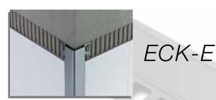
**Schluter®-ECK-E** is a stainless steel edging profile for outside corners of tiled walls that offers excellent edge protection against mechanical stresses in commercial/industrial applications. The profile produces a radiused edge along the outside wall corner for a clean, decorative finish. ECK-E is installed simultaneously with the tile.
