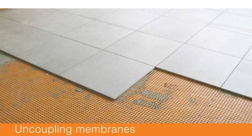
Today's construction methods, which include the use of lightweight materials, have made the installation of hard surface coverings particularly challenging. Because of the differences in material properties the substrate and the tile layer expand and contract at different rates, creating stresses in the assembly that can ultimately result in damage to the finished tile surface.
