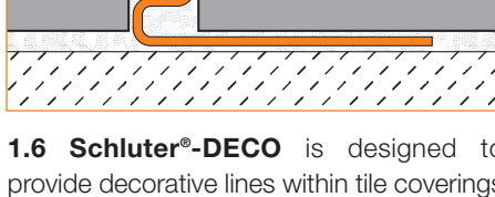
1.6 Schluter®-DECO is designed to provide decorative lines within tile coverings and edge protection at transitions from tile coverings to other same-height surface
