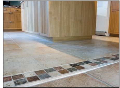
1.2 Schluter®-RENO-U , in satin nickel anodized aluminum, installed to provide a sloped transition between ceramic tile coverings at different heights. The profile produces a clean, attractive line and protects tile edges against damage.
