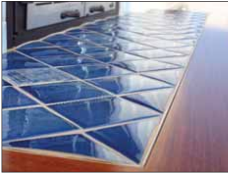
1.1 Schluter®-SCHIENE , in satin anodized aluminum, installed to protect tile edges and provide a clean transition to surrounding hardwood flooring at the same elevation.
